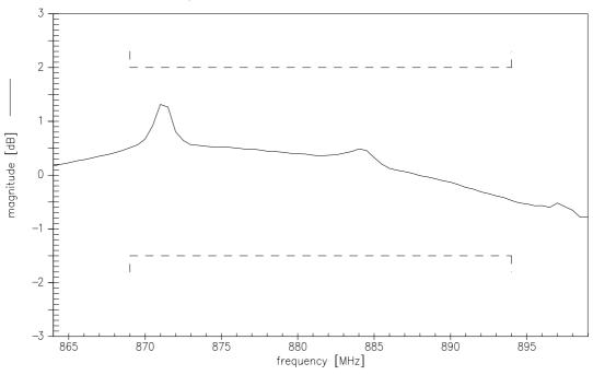
Output phase balance ( $\phi(S_{31})-\phi(S_{21})+180^{\circ}$ )
